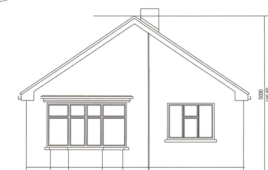
3 PROPOSED FRONT ELEVATION OF HOUSE SCALE 1:75
